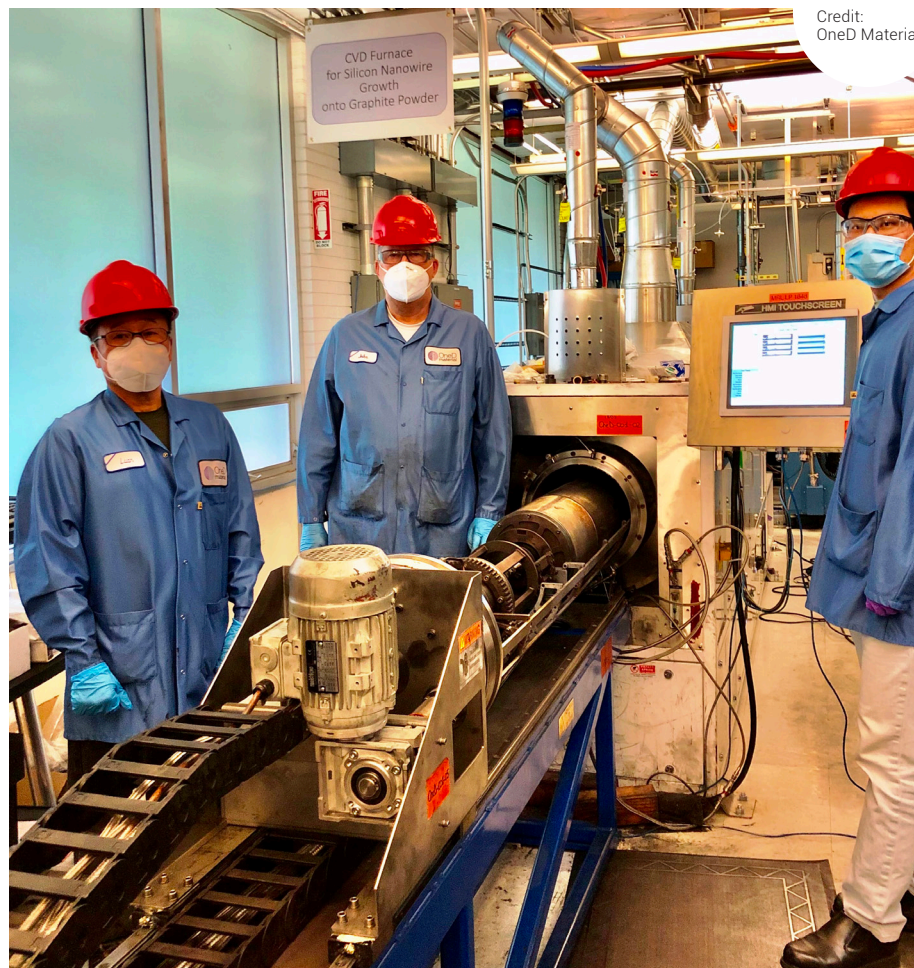
Pilot production with a single CVD process tube at OneD Material's operation in Palo Alto
